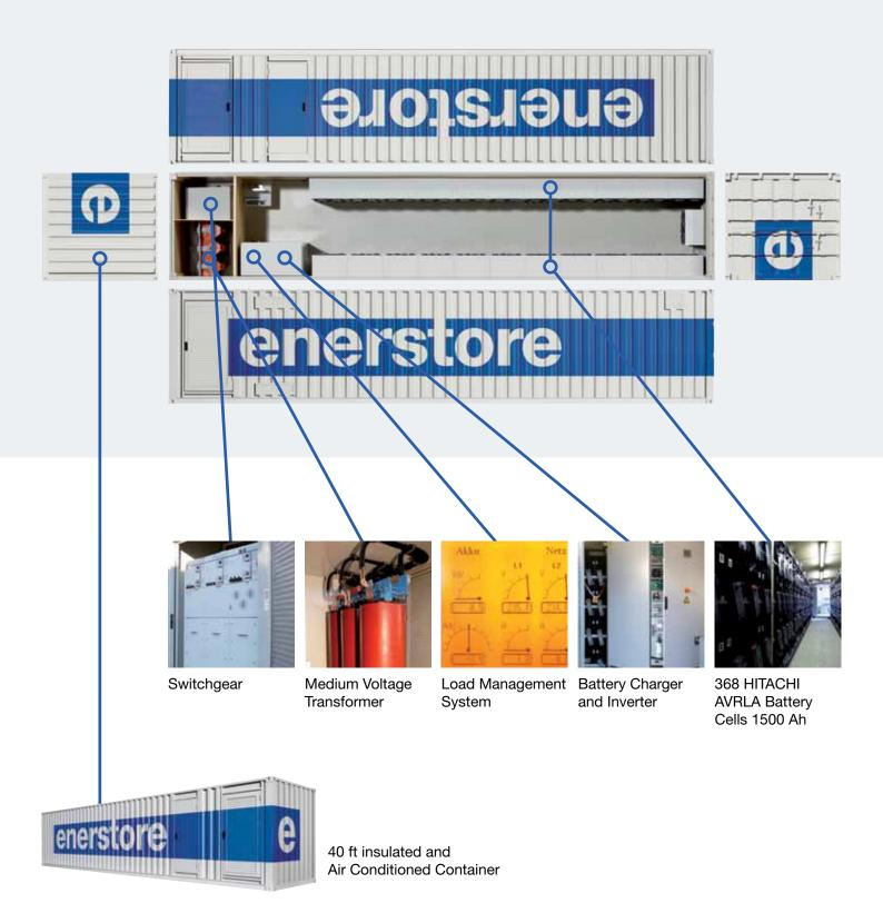
The system is supplied as a turnkey container which can be connected directly to the grid. The available energy per system is 600 – 700 kWh. Larger sizes are reached by connecting the systems in parallel.
