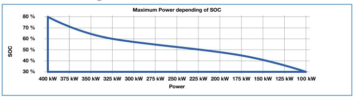
The energy storage system can be completely discharge (SOC = 30%) with a power of 100 kW. If by extracting higher power the discharge limit is reached, the remaining energy can be extracted by reducing the discharge power.
